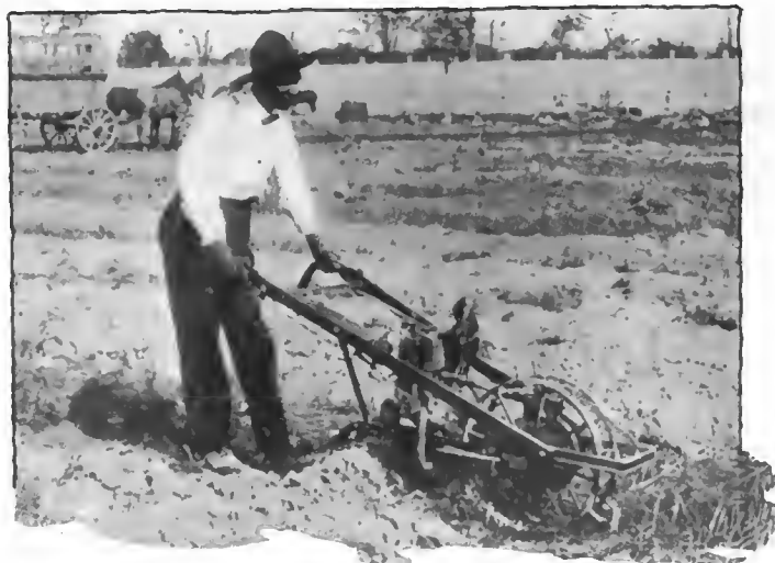
Breaking heavy wiregrass sod at the Richmond, Va., state fair with a Parker motor plow
